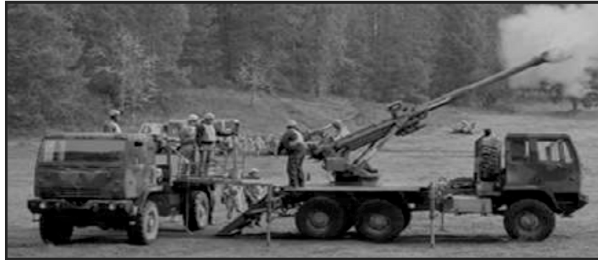
Image 2: Brutus 155 mm System (Lightweight Trails and Platform Stabilisers)
