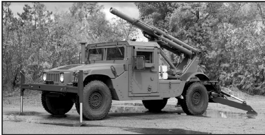
Image 1: Hawkeye: 105mm Mobile Howitzer System (Lightweight Trails and Platform Stabilisers)
